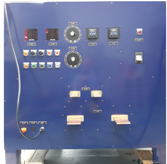
DUAL Output 15KA 3PH FWDC and 10KA AC
